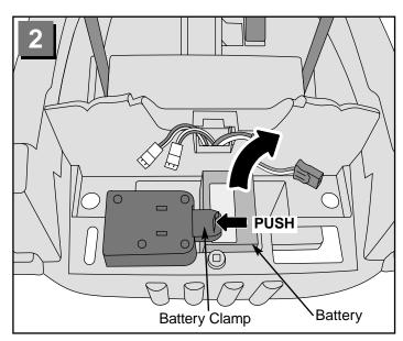
• While pushing the battery clamp, remove the battery from the vehicle body.
